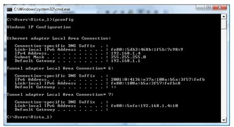
7. If an Autoconfiguration IP Address is displayed, there is an incorrect connection between the PC and the SB6120, or there are broadband network problems.
