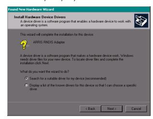
**Note**: The dialog indicates that the wizard is looking for the ARRIS RNDIS (Remote Network Device Interface Specification) driver for the Telephony Modem.
