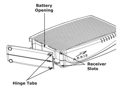
3 Push the battery pack into the bay until it latches into place. If you are taking the battery out of the Telephony Modem, use the battery pull strap to dislodge the battery.
