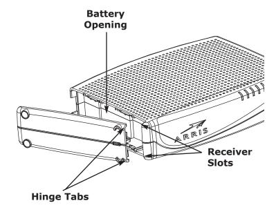
3 Push the battery pack into the bay until it seats into place. If you are taking the battery out of the Telephony Modem, position your finger in the battery opening area and use leverage to dislodge the battery while pulling it straight back.
